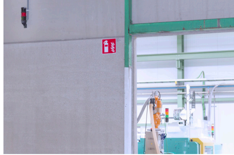
Image, left: A signal tower in the canteen indicates whether there is a machine fault, and, if so, in which area of the workshop.
