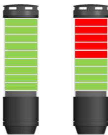
If several status warnings are active, the illuminated area is split proportionally. If the segments cannot be divided equally then the highest priority colour receives the remaining segment(s).
